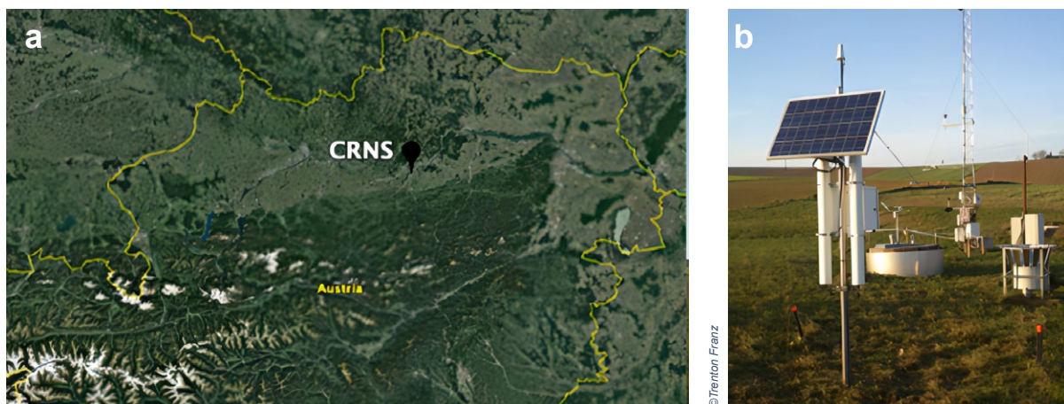
Figure 3.2. (a) Location of the CRNS (48.15°N, 15.15°E) in an agricultural area in northeast Austria; (b) CRNS located at study site with weather station and eddy covariance tower. See Figure 3.5 for raw and processed neutron counts. Source: Franz, T.E., Wahbi, A., Vreugdenhil, M., Weltin, G., Heng, L., Oismueller, M., Strauss, P., Dercon, G. & Desilets, D. 2016. Using Cosmic-ray Neutron Probes to Monitor Landscape Scale Soil Water Content in Mixed Land Use Agricultural Systems. Appl. Environ. Soil Sci. 2016. https://doi.org/10.1155/2016/432374 .
