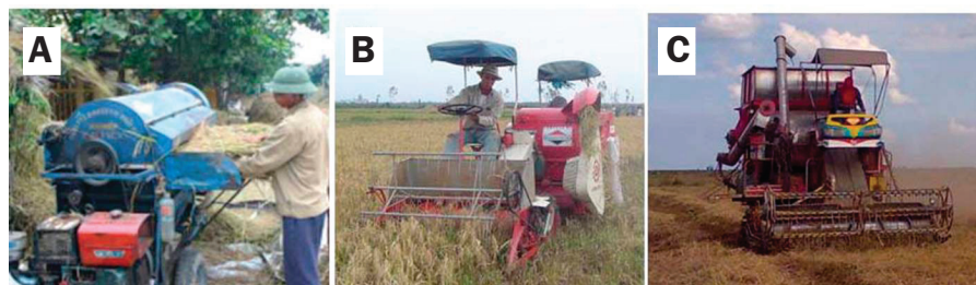
Fig. 3. (A) Axial-flow thresher in Vietnam; (B) mini combine harvester in Cambodia; (C) Thai axial-flow combine harvester.
