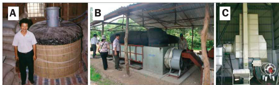
Fig. 4. (A) Low-cost farm-level dryer in Vietnam; (B) reversible air-flow batch dryer with 4-ton capacity with rice husk furnace in Vietnam; (C) re-circulating batch dryer at PhilRice, Philippines.
